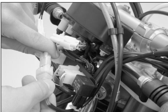
Mount the speedometer and connect the Tripmaster switch. Mount the headlight mask.
