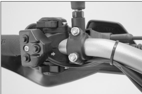
Tighten the screws and run the wiring harness parallel to the light switch wiring harness under the headlight mask.
