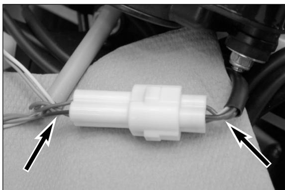
To sever, remove the headlight mask and sever the black cable on the speedometer wiring harness or the black/brown cable on the vehicle wiring harness. Insulate both ends with insulating tape and remount the headlight mask. You can reinstate the original condition by connecting the wires again.
