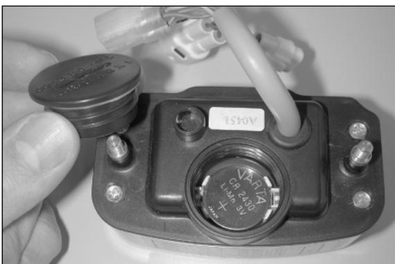
Remove the headlight mask and disassemble the electronic speedometer. Remove the screw connection ❷, insert the supplied battery (type Duracell CR 2430) with the writing facing up and reinstall the screw connection.
